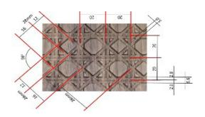
Besides the allowance of +/-0,3 mm of the total area thickness referring to the highest point there are minor differences in the thickness of the embossment - with a max. of 1.3 mm due to the natural design specifications.
