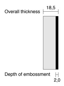
Besides the allowance of +/-0,3 mm of the total area thickness referring to the highest point there are minor differences in the thickness of the embossment - about 2,0 mm due to the natural design specifications.
